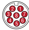
Integral D84 connector (male) as viewed from the end of the sensor
