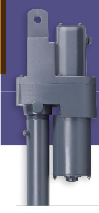
Joyce linear actuators are designed to lift and precisely position loads of up to 1500 pounds. They are built with cast aluminum housings, include motors (120 VAC or 12 VDC), and are best suited for use in environments that are protected from the elements. A spring brake ensures that the actuators hold position when power is off. The maximum speed, which varies with load, is about 50 inches per minute (LA155).
